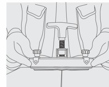
After scoring the length and making the cut, move the slab out of the workbench till the incision line and split from both sides using cutting-off pliers.
