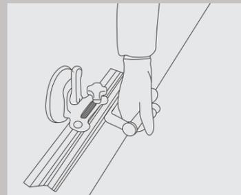
Ensure proper suction with a vacuum between the device and the slab and use a single device/suction cup for a maximum length of up to 150cms.
