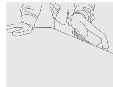
Smooth the edges of the length cut with a diamond polishing pad.
