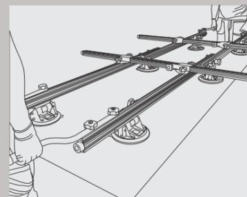
To lift the slabs use sucker cups after cleaning the slab and cups with a damp sponge. Make sure the device also has suckers that run along with the guides and adhere to the slab.
