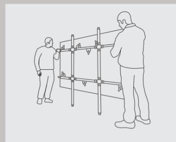
To lift the slab use guides from the long sides of the slab and lift/hang it vertically to the handles of the trolley frame. Use appropriate size reinforced trolley for various sizes of slabs.
